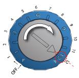
Rotary switch for discharge period setting
